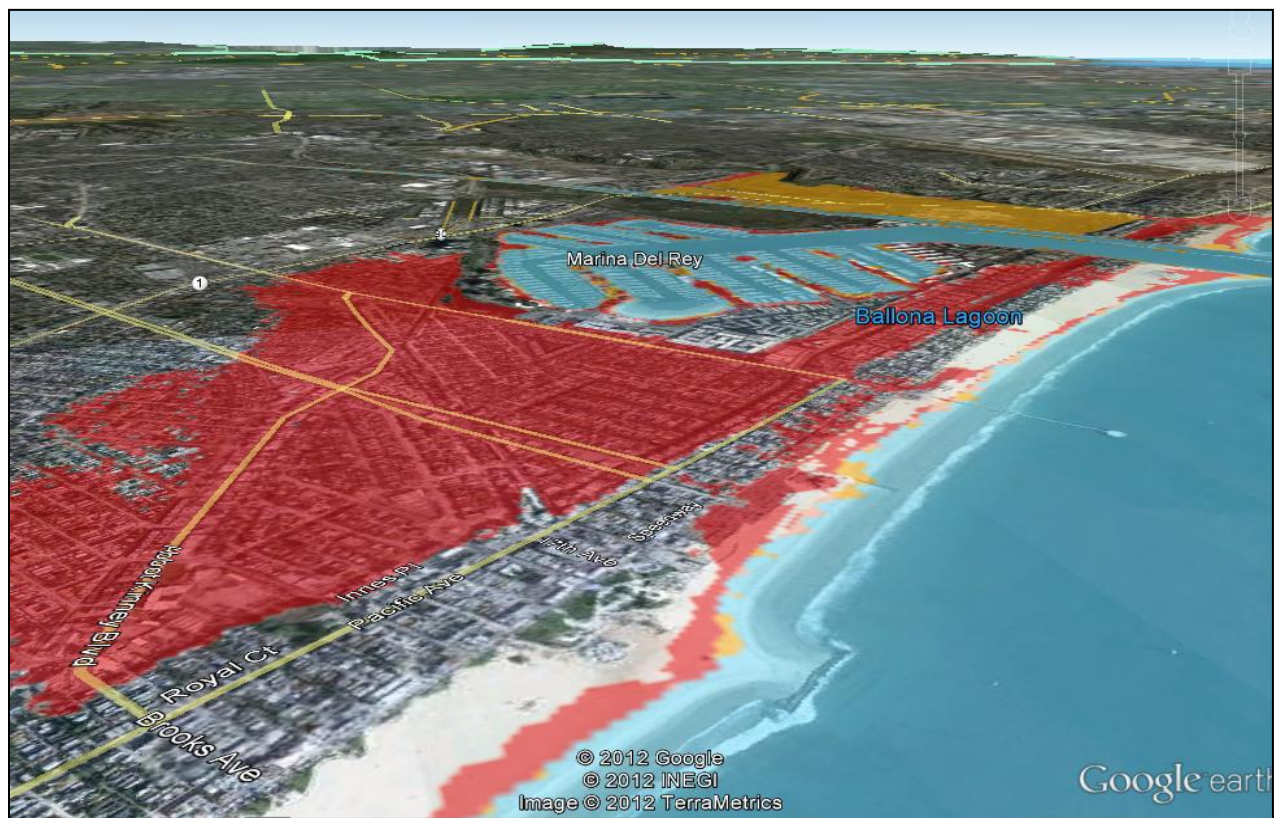
FIGURE 9. EXTENT OF FLOODING IN VENICE FROM SEA-LEVEL RISE (ORANGE REPRESENTS 16 INCHES AND RED REPRESENTS 55 INCHES OF SEA-LEVEL RISE), AS MODELED BY USGS (BARNARD 2012) 36 UNDER A 10 YEAR STORM. ADDITIONAL LAND WOULD BE AT RISK OF FLOODING DURING A 100 YEAR STORM. LARGE PORTION IN ORANGE COVERS BALLONA WETLANDS
