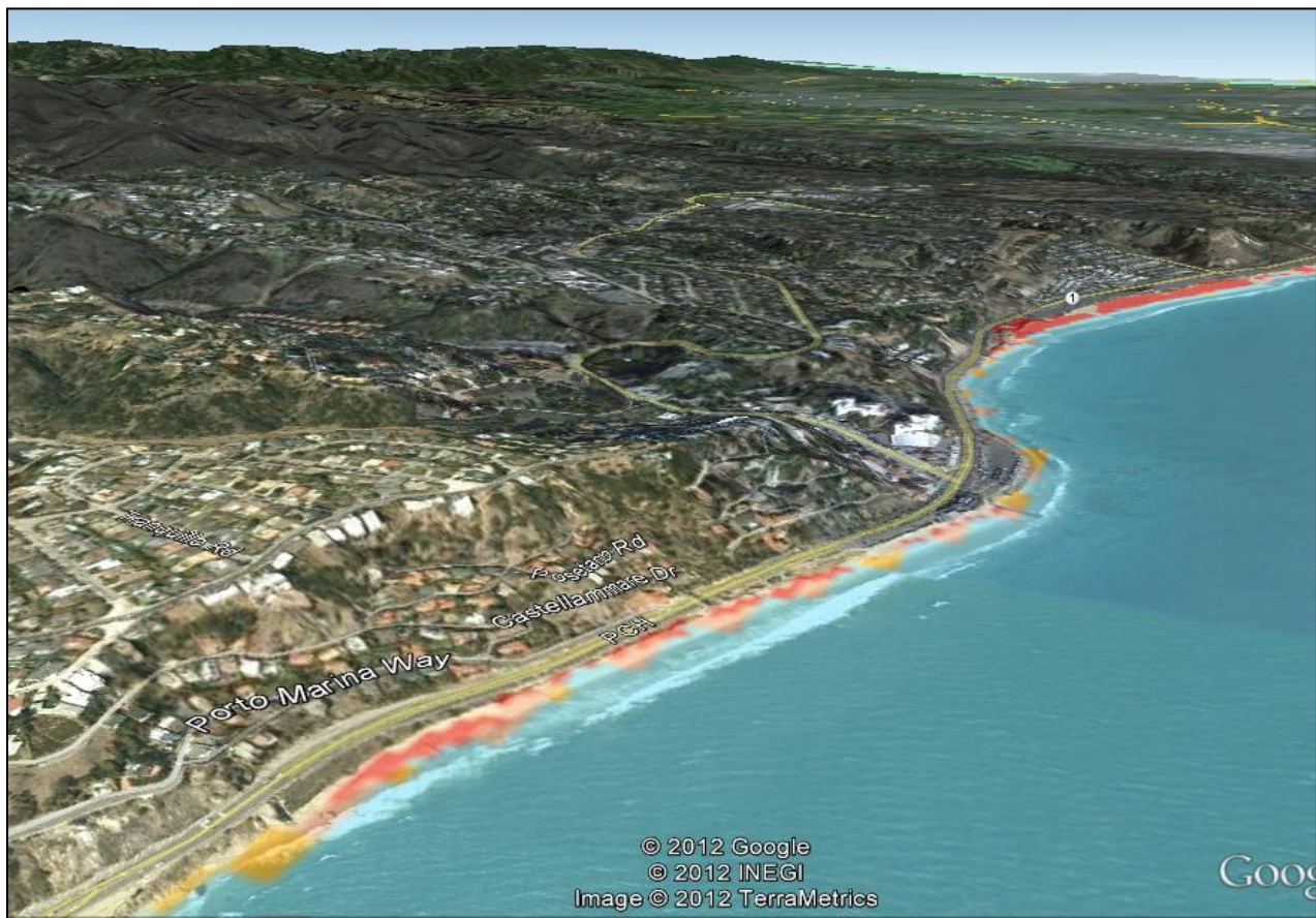
FIGURE 7. EXTENT OF FLOODING ALONG THE SHORELINE OF PACIFIC PALISADES IN A 10-YEAR FLOOD WITH SEA-LEVEL RISE OF 16 INCHES (ORANGE) AND 55 INCHES (RED). SOURCE: BARNARD USGS 2012.
